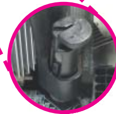
"Unlocked" position of push-pin
